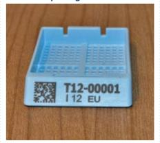
Confusions and mix ups are nearly fully eradicated and searching for the right labels is over! The cassettes can be scanned by the microtome with a 2D-barcode on the cassette itself, after which label printers or glass printers print out the requests. The module is also available for (room-saving) touchscreen PCs.
