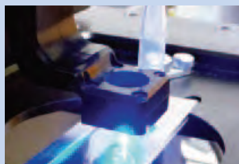
2. A single dehydrated brain tissue section mounted on top of a MMI MembraneSlide.
